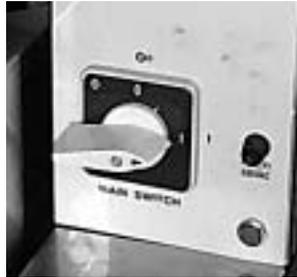
2. Turn on Motor Power Switch and set Motor Speed Control to desired setting. (Use a setting of "50" to start.)
