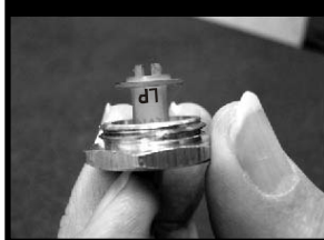
6. Note you can read LP on the plastic part it is now in the LP position
