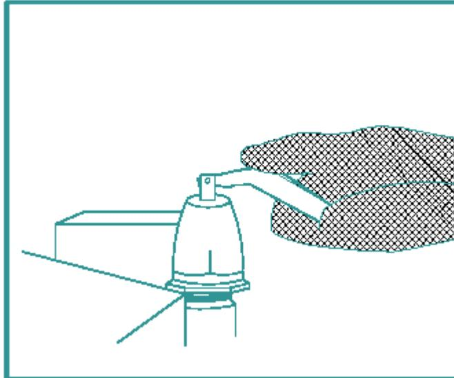
2. Release the lever on the valve, and let it slam shut to seal the valve.
