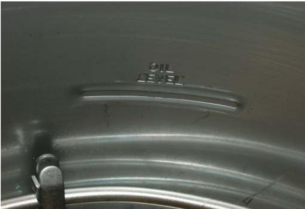
2. Place the **FILTER/OFF/FRY** switch to the **FRY** position. The shortening should begin to heat and begin to reach the fill mark inside the pot. Add more shortening as required to reach the fill mark. Refer to the troubleshooting section if this does not occur.
