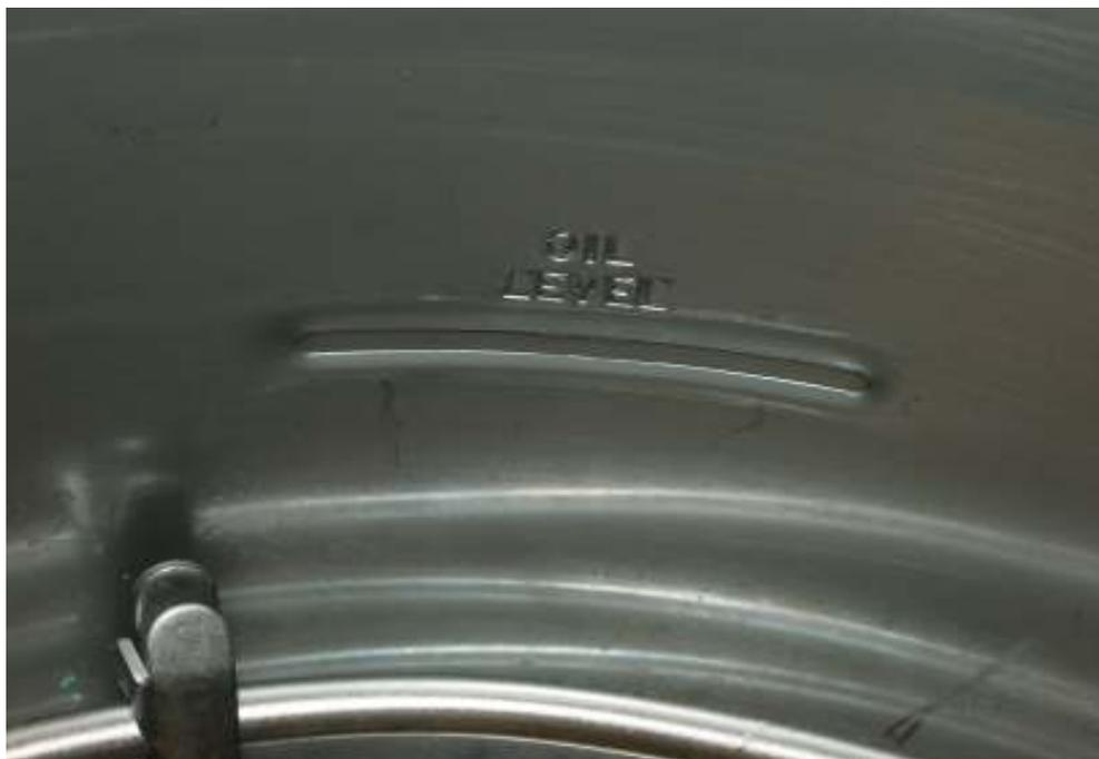
3. Place the **FILTER/OFF/FRY** switch to the **FRY** position. The question "Is the Fry Pot filled – If yes press ENTER" will appear on the computer display. The shortening will heat and begin to reach the fill mark inside the pot.
