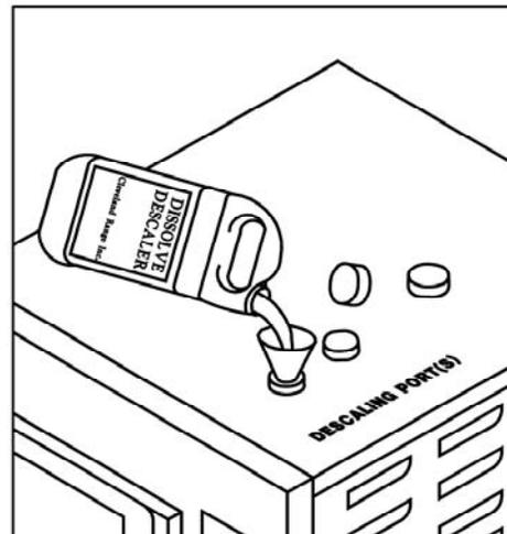
Figure 6-1 Descaling Port
