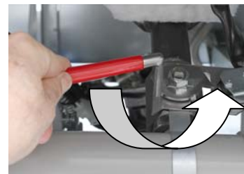
Move the red drain valve handle into the open position (right).
