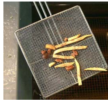
Prior to filtering, skim any large debris from oil in frypot.
