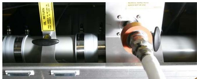
The handle (right above) next to the oil-disposal quick-disconnect activates the filter pump. All drain valves should be closed when oil is being pumped out for disposal.
