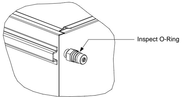
5. Push the prepared filter pan back into the fryer cabinet and reconnect the suction hose to the pan.
