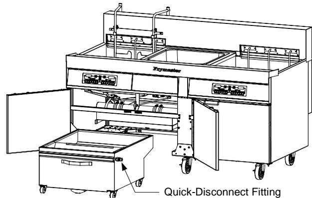
2. Remove the crumb screen, hold-down ring, filter paper, and filter grid from the pan. Dispose of the filter paper, clean all other components in hot, soapy water and dry thoroughly. Clean the pan and sump, ensuring the air hole in the pickup (suction) tube is clear of debris.
