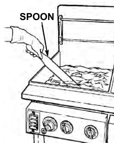
FIGURE 5. STIR WITH SPOON PROVIDED TO REMOVE WATER
