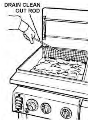
FIGURE 4. REMOVE SCREEN OVER TUBES/ELEMENTS
