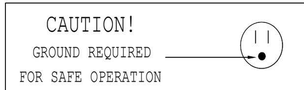
*This label is located on top of the electrical control on models with a power cord.*
