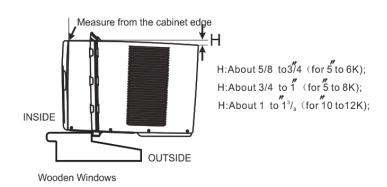
NOTE: Check that air conditioner is tilted back about H(tiled about  $3^{\circ}$  to  $4^{\circ}$  downward to the outside). After proper installation, condensate should not drain from the overflow drain hole during normal use, correct the slope otherwise.
