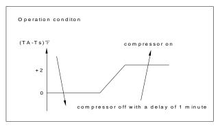
When TA≤TS, compressor off When T1>TS+2°F, compressor on
