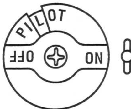
Fig. 10 "On" position on Unitrol (Fryers with standing pilot ignition)
