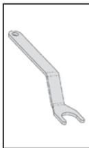
**A special tool** has also been designed to **remove** this hollowing nut.
