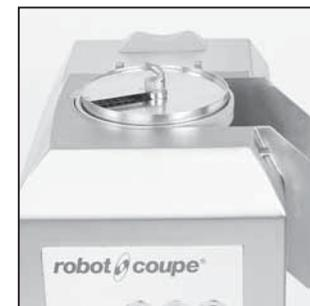
4) Position the pusher feed head on the motor base. The fastening hook should now be facing you, on your right.
