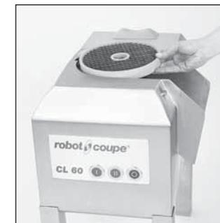
Fit the dicing grid over the motor shaft. As shown in the picture, the grid rests on a ledge in the motor base.
