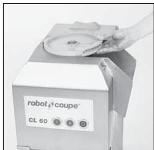
ledge must be clean and free of product in order for the machine to operate correctly. **Make sure the plastic tab on the outer rim of the grid is fully seated in the corresponding slot in the motor unit.** The cutting blades on the grid should be facing the exit chute.
