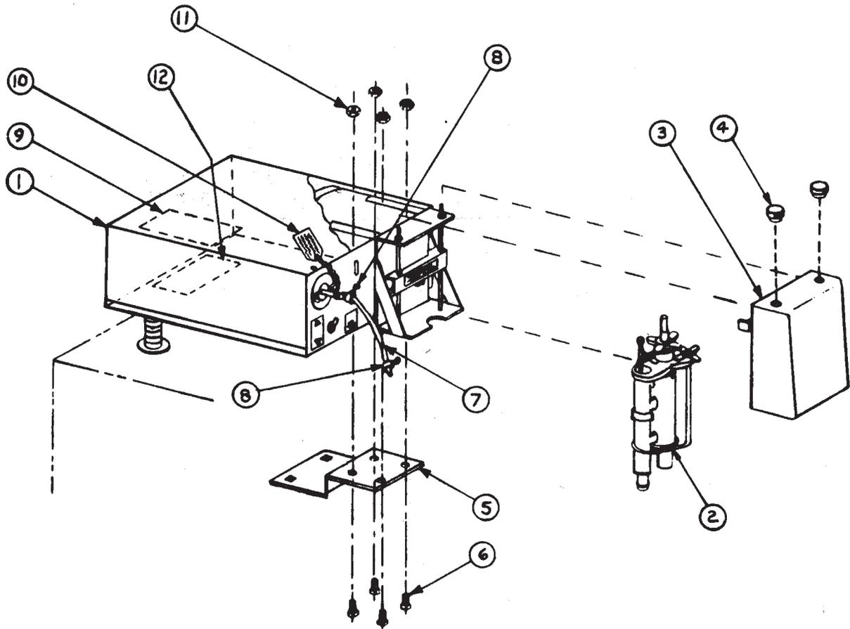
Figure 16. Hopper Pump Final Assembly
