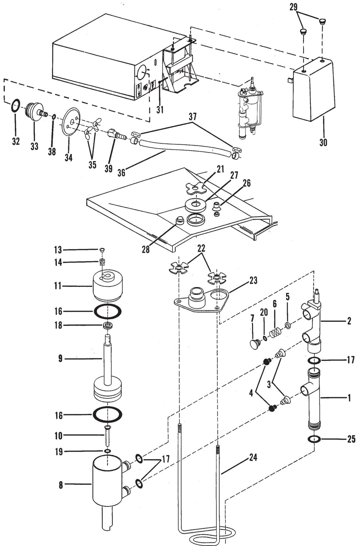
Figure 17. Mix Pump Parts
