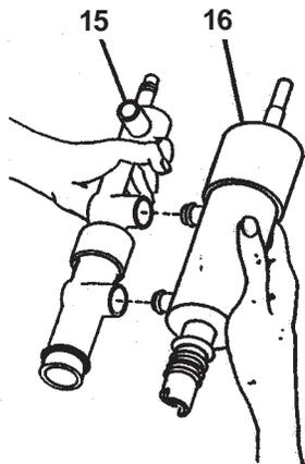
**Figure 8. Pump Disassembly Step Two**
