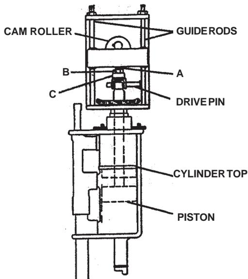
Figure 14. Over-Run Adjustment
