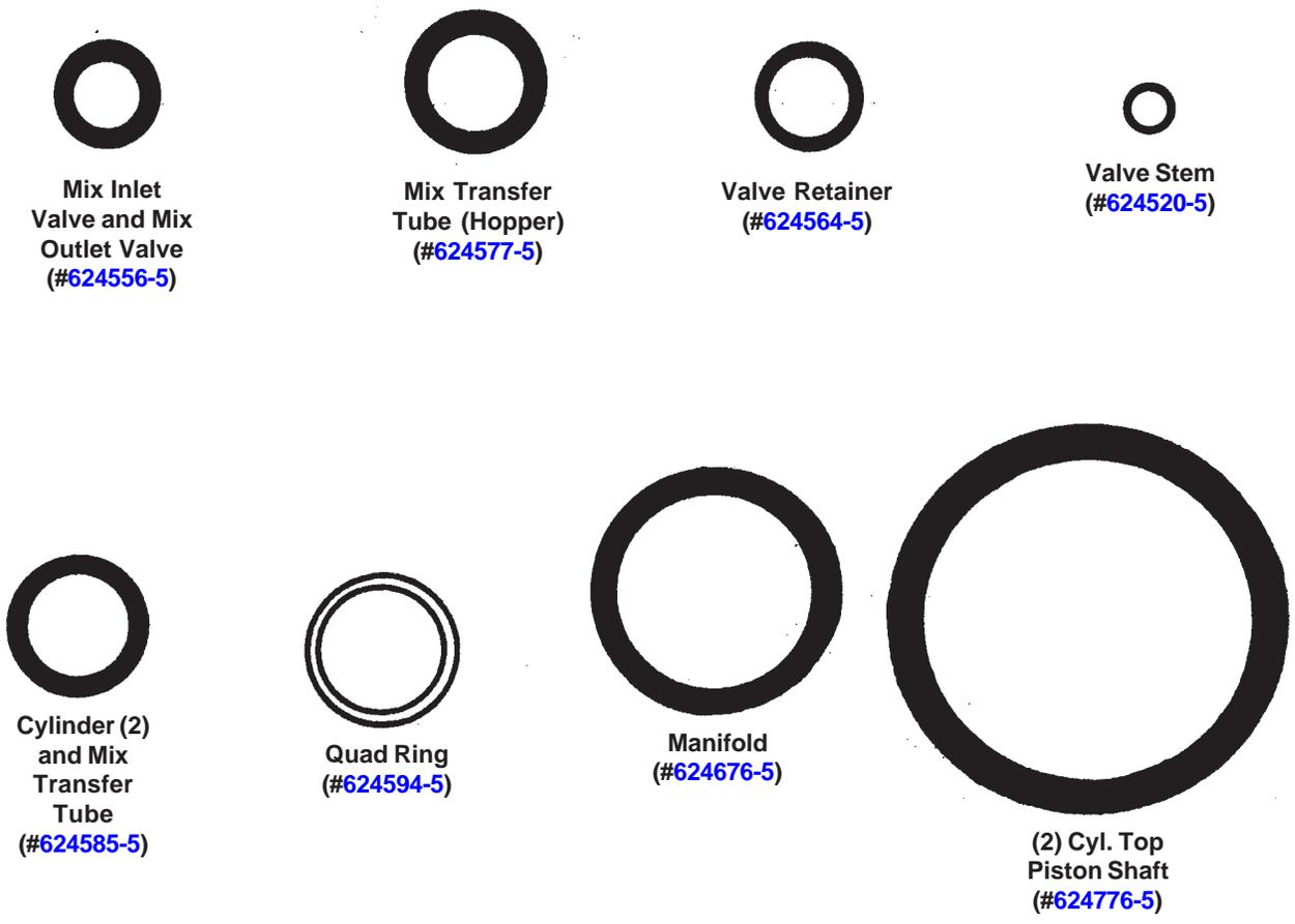
Figure 13. "O"-Ring Identification (Actual Size)
