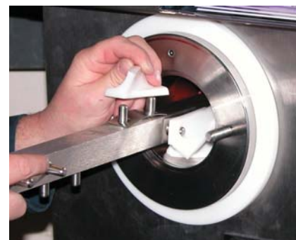
Figure 3-6 Installing Auger Blades
