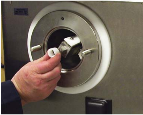
Figure 3-7 Install Front Wear Bushing
