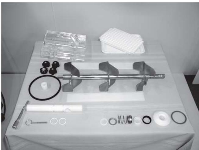
**Figure 7. Front Door and Auger Assembly**
