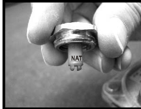
7. Replace the brass cap back into the body of the regulator
