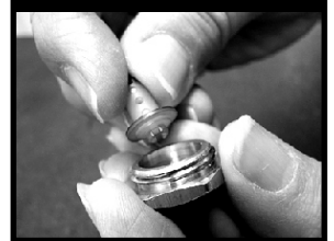
4. Snap the plastic part off of the brass cap
