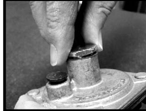
7. Replace the brass cap back into the body of the regulator
